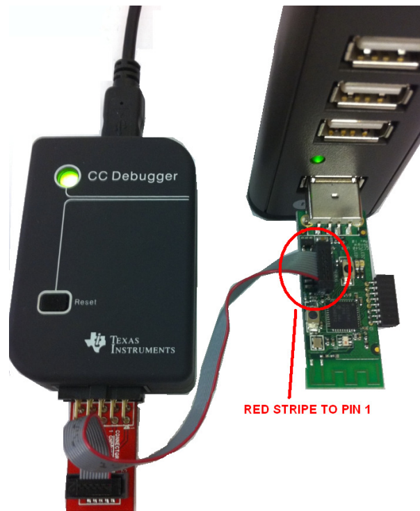
Figure 29 CC2540 USB Dongle Connected to CC Debugger
