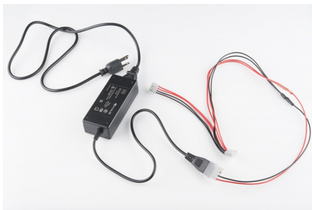
Finished panel power supply cable.
