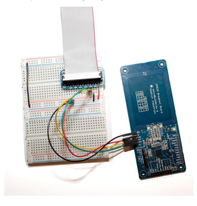
**Note:** Make sure that the **SELO** and **SEL1** jumpers on the NFC breakout are set to **OFF**, which will cause the PN532 to boot into UART mode (rather than SPI and I2C, which aren't currently supported by libnfc). You will need to reset the breakout after changing these pins, which you can do by cycling the power pin.
