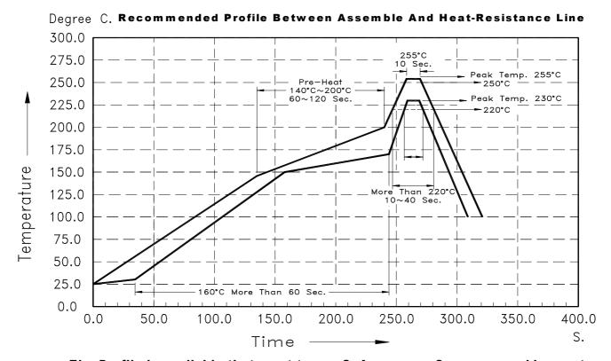
The Profile is available that must to use SnAg  $_{(x=3.3\sim3.8)}$  Cu  $_{(y=0.2\sim0.7)}$  solder paste
