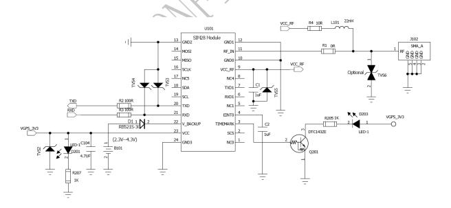
Figure 12: Example application schematic
