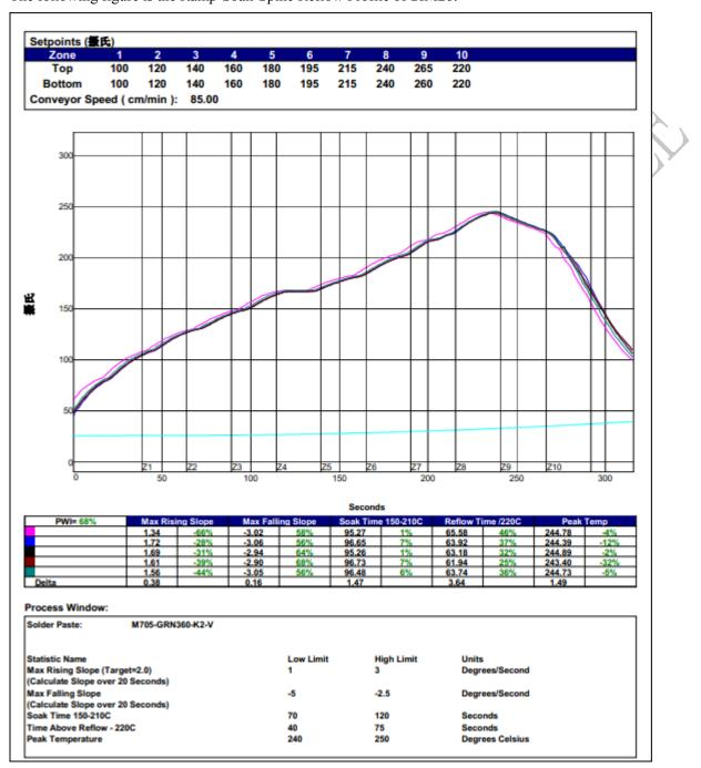
Figure 11: The Ramp-Soak-Spike reflow profile of SIM28
