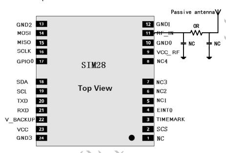
Figure 6: SIM28 passive antenna design
