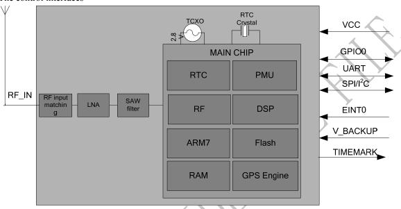
Figure 1: SIM28 functional diagram
