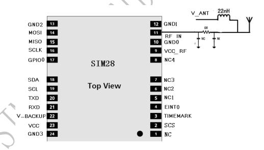
Figure 9: SIM28 Active antenna design
