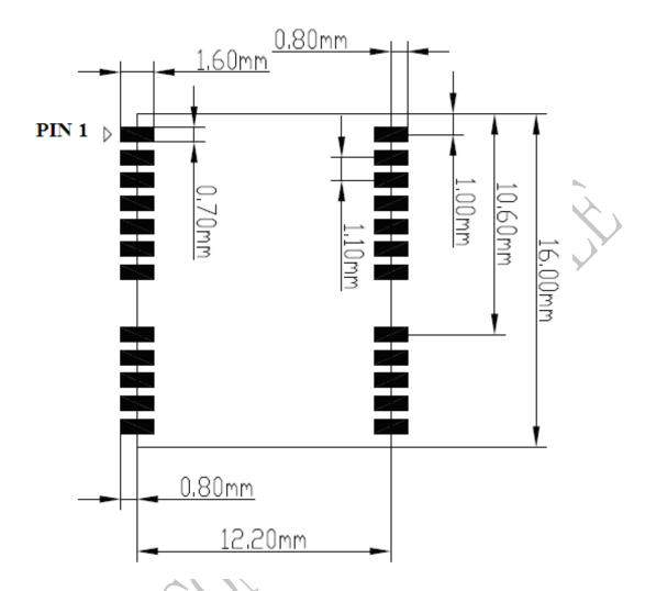
Figure 4: Recommended PCB decal (top view) (Unit: mm)
