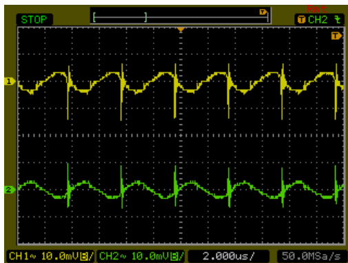
Typical Output Ripple and Noise. V_{in} = V_{in\ nom} ; Full Load; T_A
