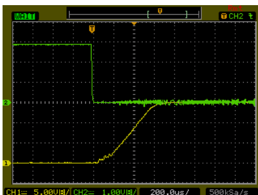
Using ON/OFF Voltage Start-Up and V_{out} Rise Characteristic V_{in} = V_{in\ nom} ; Full Load
