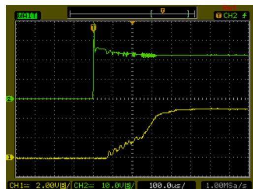
Typical Input Start-Up and Output Rise Characteristic
