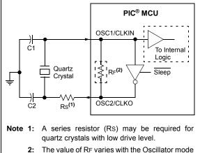
2: The value of RF varies with the Oscillator mode selected (typically between 2 M $\Omega$  to 10 M $\Omega$ ).
