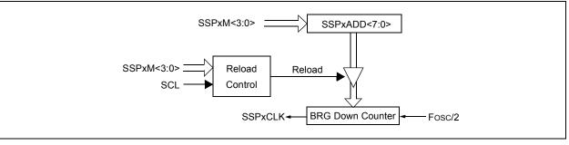
Note: Values of 0x00, 0x01 and 0x02 are not valid for SSPxADD when used as a Baud Rate Generator for I<sup>2</sup>C<sup>™</sup>. This is an implementation limitation.
