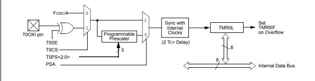
Note: Upon Reset, Timer0 is enabled in 8-bit mode with clock input from T0CKI max. prescale.
