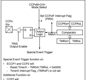
Set ADCON0<1>, GO/DONE bit to start an ADC Conversion if ADCON<0>, ADON = 1, and if ADCON1<7>. TRIGSEL = 0.
