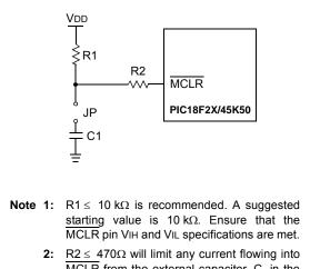
MCLR from the external capacitor, C, in the event of MCLR pin breakdown, due to Electrostatic Discharge (ESD) or Electrical Overstress (EOS). Ensure that the MCLR pin VIH and VIL specifications are met.
