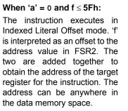
Note that in this mode, the correct syntax is now: ADDWF [k], d where 'k' is the same as 'f'.
