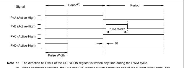
2: When changing directions, the PxA and PxC signals switch before the end of the current PWM cycle. The modulated PxB and PxD signals are inactive at this time. The length of this time is (Timer2 Prescale)/Fosc.
