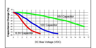
When selecting a ceramic capacitor to be used with the internal voltage regulator, it is suggested to select a high-voltage rating, so that the operating voltage is a small percentage of the maximum rated capacitor voltage. For example, choose a ceramic capacitor rated at 16V for the 3.3V VUSB3V3 voltage.
