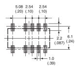
Terminal Arrangement/ Internal Connections (Bottom view)
