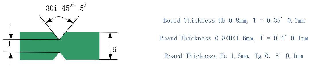
Figure 3: Board thickness requirements for v-cut scoring.
