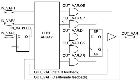
OUT\_VAR.D = IN\_VAR1 & OUT\_VAR # !IN\_VAR2 & IN\_VAR3.DQ # !IN\_VAR1 & OUT\_VAR.IO
