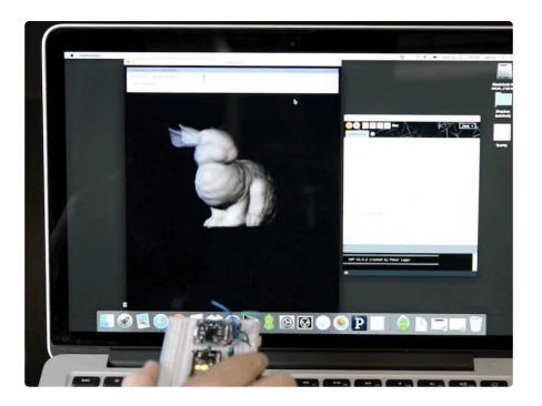
Also notice in the upper right corner of the dialog box at the top that the calibration of each sensor is displayed. It's important to calibrate the BNO055 sensor so that the most accurate readings are retrieved. Each sensor on the board has a separate calibration status from 0 (uncalibrated) up to 3 (fully calibrated). Check out the <u>video</u> and information from this guide for how to best calibrate the BNO055 sensor (https://adafru.it/kA1).
