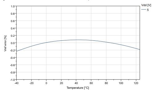
Figure 39-31. Internal 4.3V Reference vs. Temperature
