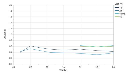
Figure 39-50. DNL vs.  $V_{REF}$  ( $V_{DD}$ =5.0V,  $f_{ADC}$ =115 ksps, REFSEL = External Reference)
