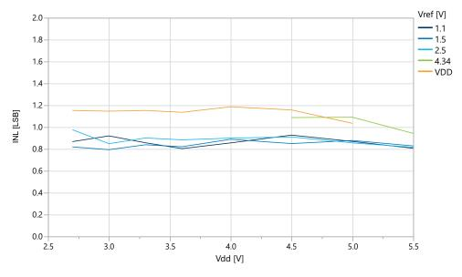
Figure 39-44. INL vs.  $V_{ref}$  ( $V_{DD}$ =5.0V,  $f_{ADC}$ =115 ksps), REFSEL = Internal Reference
