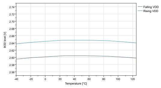
Figure 39-36. BOD Threshold vs. Temperature (Level 4.3V)
