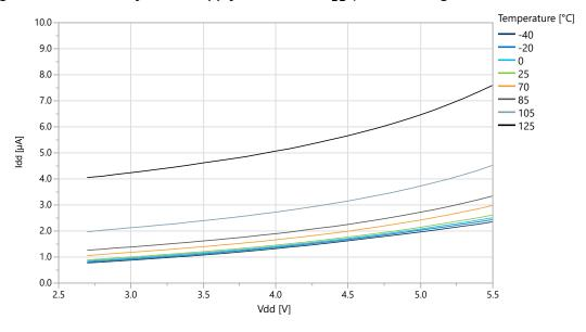
Figure 39-14. Standby Mode Supply Current vs. V<sub>DD</sub> (Sampled BOD Running at 125 Hz)
