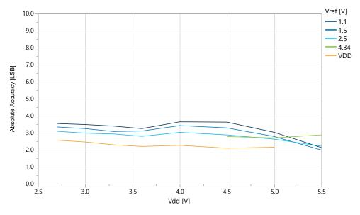
Figure 39-38. Absolute Accuracy vs.  $V_{ref}$  ( $V_{DD}$ =5.0V,  $f_{ADC}$ =115 ksps), REFSEL = Internal Reference
