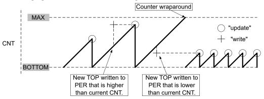
A counter wraparound can occur in any mode of operation when up-counting without buffering. This is due to the fact that the TCAn.CNT and TCAn.PER registers are continuously compared: if a new TOP value is written to TCAn.PER that is lower than current TCAn.CNT, the counter will wrap first, before a compare match happens.
