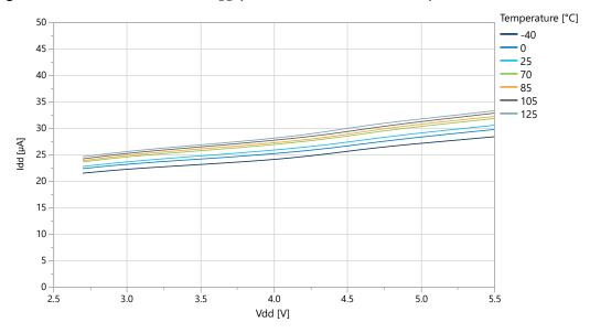
Figure 39-33. BOD Current vs. V<sub>DD</sub> (Sampled BOD at 125 Hz)
