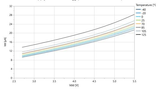
Figure 39-5. Active Supply Current vs. V<sub>DD</sub> (f=32 KHz OSCULP32K)
