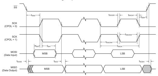
Table 38-17. USART in SPI Master Mode - Timing Characteristics
