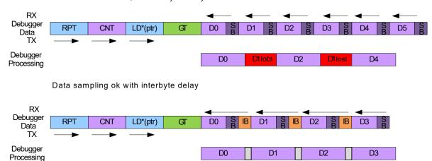
In Figure 34-18, GT denotes the Guard Time insertion, SB is for Stop Bit and IB is the inserted interbyte delay. The rest of the frames are data and instructions.
