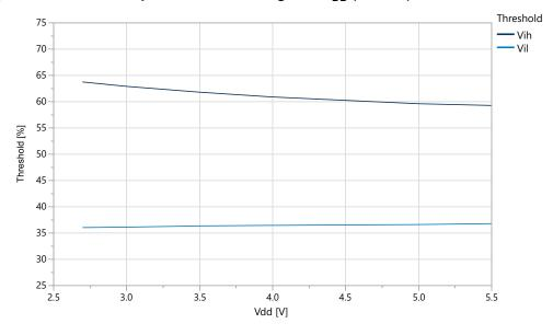
Figure 39-18. I/O Pin Input Threshold Voltage vs.  $V_{DD} (V_{IH})$
