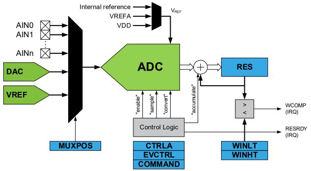
The analog input channel is selected by writing to the MUXPOS bits in the MUXPOS register (ADC.MUXPOS). Any of the ADC input pins, GND, can be selected as single-ended input to the ADC. The ADC is enabled by writing a '1' to the ADC ENABLE bit in the Control A register (ADC.CTRLA). Voltage reference and input channel selections will not go into effect before the ADC is enabled. The ADC does not consume power when the ENABLE bit in ADC.CTRLA is '0'.
