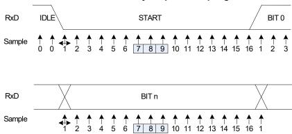
The transmission baud rate must be set up in relation to the selected UPDI clock, which can be adjusted by UPDICLKSEL in UPDI.ASI\_CTRLA. See Table 34-2 for recommended maximum and minimum baud rate settings.
