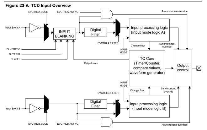
There is a delay of 2-3 clock cycles on the TCD synchronizer clock between receiving the input event, processing it, and overriding the outputs. If using the asynchronous event detection, the outputs will override instantly outside the input processing.
