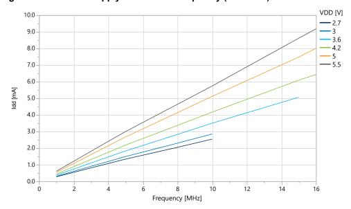
Figure 39-2. Active Supply Current vs. Frequency [0.1, 1.0] MHz at T=25°C
