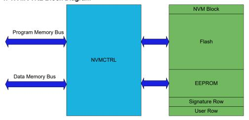
**Nonvolatile Memory Controller (NVMCTRL)**
