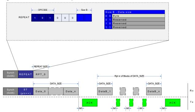
The figure above gives an example of repeat operation with an ST instruction using pointer post-increment operation. After the REPEAT instruction is sent with RPT\_0 =  $\boldsymbol{n}$ , the first ST instruction is issued with SYNCH and Instruction frame, while the next  $\boldsymbol{n}$  ST instructions are executed by only sending in data bytes according to the ST operand DATA\_SIZE, and maintaining the Acknowledge (ACK) handshake protocol.
