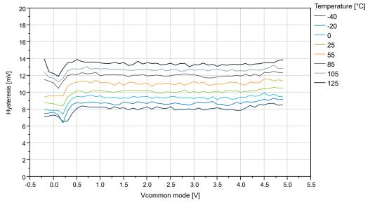
Figure 39-58. Hysteresis vs.  $V_{CM}$  - 10 mV to 50 mV ( $V_{DD}$ =5V, T=25°C)
