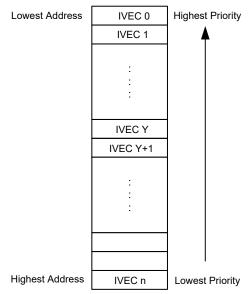
The default priority can be changed by writing to the CPUINT.LVL0PRI register. The value written to the register will identify the vector number with the lowest priority. The next interrupt vector in IVEC will have the highest priority, see the following figure. In this figure, the value Y has been written to
