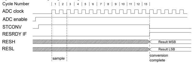
Both sampling time and sampling length can be adjusted using the Sample Delay bit field in Control D (ADC.CTRLD) and sampling the Sample Length bit field in the Sample Control register (ADC.SAMPCTRL). Both of these control the ADC sampling time in a number of CLK\_ADC cycles. This allows sampling high-impedance sources without relaxing conversion speed. See the register description for further information. Total sampling time is given by:
