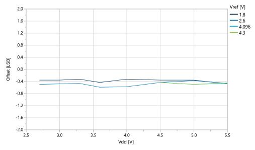
Figure 39-56. Offset vs. V<sub>REF</sub> (V<sub>DD</sub>=5.0V, f<sub>ADC</sub>=115 ksps, REFSEL = External Reference)
