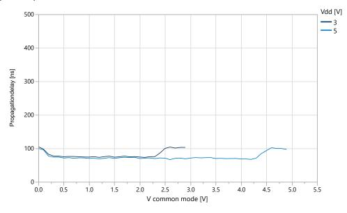
Figure 39-62. Propagation Delay vs.  $V_{CM}$  LPMODE Enabled, Rising Positive Input,  $V_{OD}$  = 30 mV (T=25°C)
