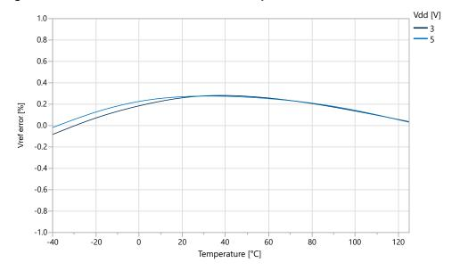
Figure 39-30. Internal 2.5V Reference vs. Temperature
