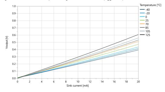
Figure 39-22. I/O Pin Output Voltage vs. Sink Current (T=25°C)
