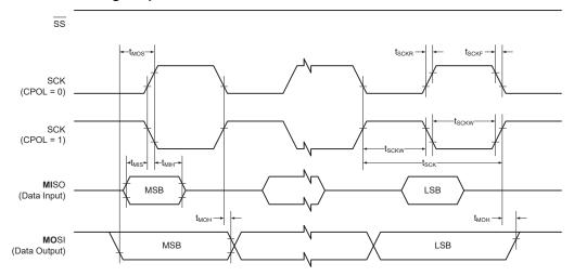
Figure 38-6. SPI - Timing Requirements in Slave Mode
