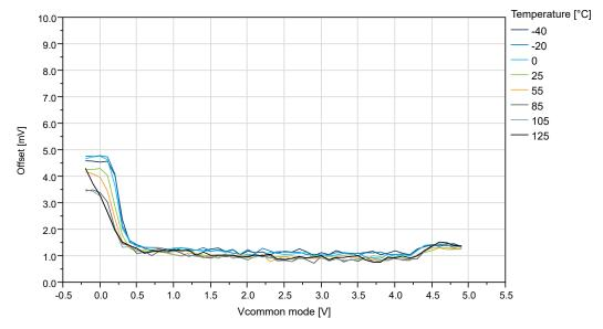
Figure 39-60. Offset vs.  $V_{CM}$  - 10 mV to 50 mV ( $V_{DD}$ =5V, T=25°C)
