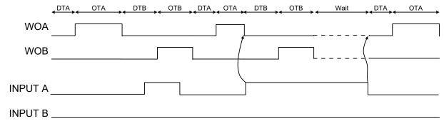
If Input mode 2 is used on input B, an event will only have an effect if the TCD is in Dead-time B or On-time B, and it will only affect the output WOB.
