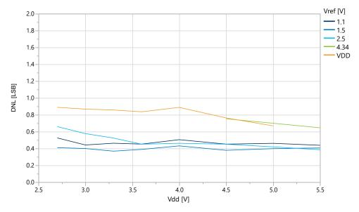
Figure 39-40. DNL vs.  $V_{ref}$  ( $V_{DD}$ =5.0V,  $f_{ADC}$ =115 ksps), REFSEL = Internal Reference
