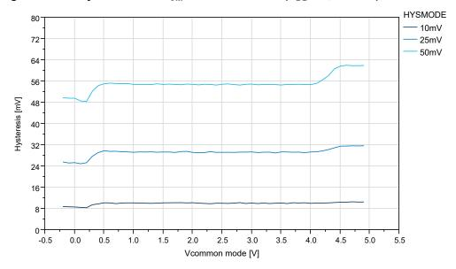
Figure 39-59. Offset vs.  $V_{CM}$  - 10 mV ( $V_{DD}$ =5V)
