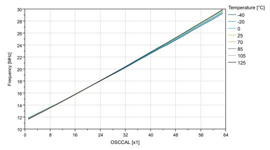
Figure 39-67. OSC20M Internal Oscillator: Frequency vs. Temperature
