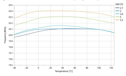
Figure 39-68. OSC20M Internal Oscillator: Frequency vs.  $V_{DD}$
