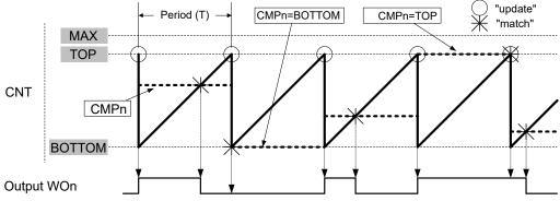
The TCAn.PER register defines the PWM resolution. The minimum resolution is 2 bits (TCA.PER=0x0003), and the maximum resolution is 16 bits (TCA.PER=MAX).
