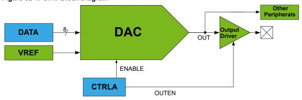
**Note:** Only DAC0 has an output driver for an external pin.
