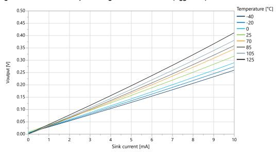
Figure 39-21. I/O Pin Output Voltage vs. Sink Current (V<sub>DD</sub>=5.0V)
