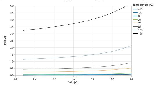
Figure 39-11. Power-Down Mode Supply Current vs. V<sub>DD</sub> (all functions disabled)
