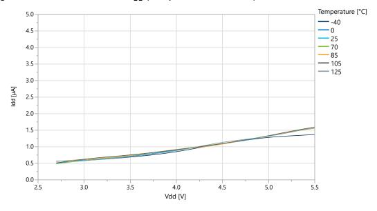
Figure 39-34. BOD Current vs. V<sub>DD</sub> (Sampled BOD at 1 kHz)
