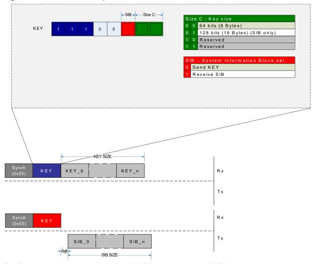
The figure above shows the transmission of a KEY and the reception of a SIB. In both cases, the  $SIZE\_C$  field in the opcode determines the number of frames being sent or received. There is no response after sending a KEY to the UPDI. When requesting the SIB, data will be transmitted from the UPDI according to the current Guard Time setting.
