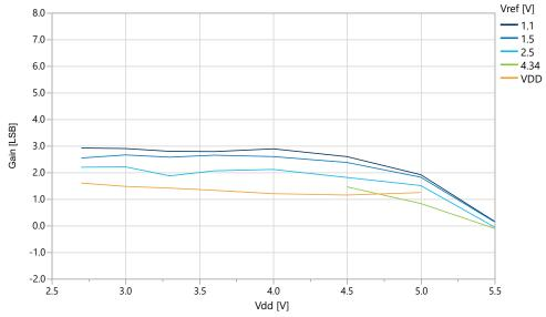
Figure 39-42. Gain Error vs.  $V_{ref}$  ( $V_{DD}$ =5.0V,  $f_{ADC}$ =115 ksps), REFSEL = Internal Reference
