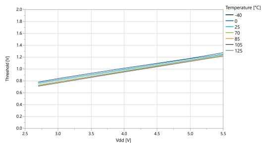
Figure 39-17. I/O Pin Input Threshold Voltage vs. V<sub>DD</sub> (T=25°C)
