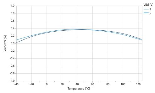
Figure 39-29. Internal 1.1V Reference vs. Temperature
