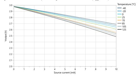
Figure 39-24. I/O Pin Output Voltage vs. Source Current (V<sub>DD</sub>=5.0V)
