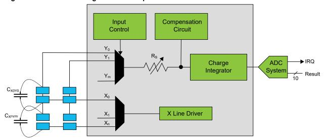
Figure 33-2. PTC Block Diagram Self Capacitance
