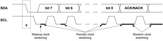
**Note:** Clock stretching is not supported by all I<sup>2</sup>C slaves and masters.
