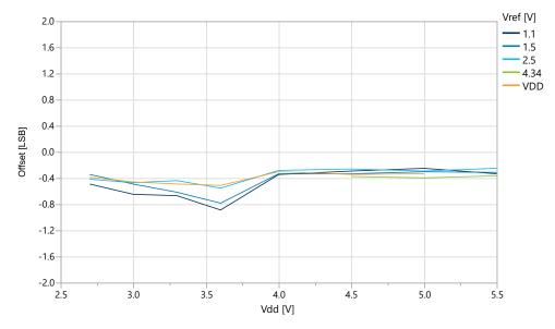
Figure 39-46. Offset Error vs.  $V_{ref}$  ( $V_{DD}$ =5.0V,  $f_{ADC}$ =115 ksps), REFSEL = Internal Reference
