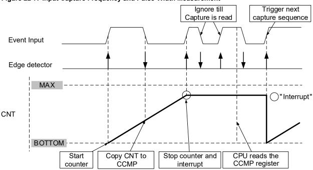
Figure 22-7. Input Capture Frequency and Pulse-Width Measurement
