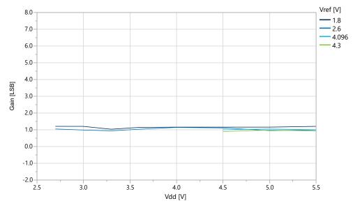
Figure 39-52. Gain vs.  $V_{REF}$  ( $V_{DD}$ =5.0V,  $f_{ADC}$ =115 ksps, REFSEL = External Reference)
