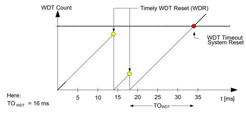
Normal mode is enabled as long as the WINDOW bit field in the Control A register (WDT.CTRLA) is 0x0.
