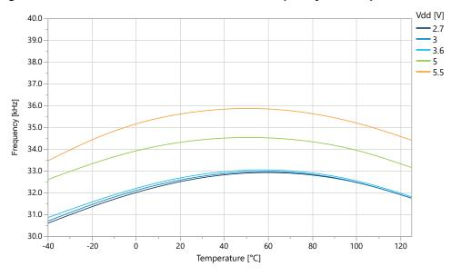
Figure 39-70. OSCULP32K Internal Oscillator Frequency vs. V<sub>DD</sub>
