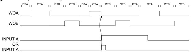
If Input mode 8 is used on input B and a positive input event occurs while in On-time B, the TCD counter jumps to Dead-time A.
