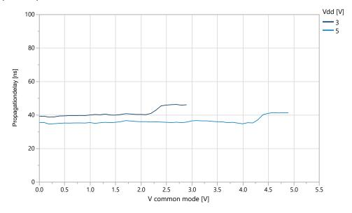
Figure 39-64. Propagation Delay vs.  $V_{CM}$  LPMODE Disabled, Rising Positive Input,  $V_{OD}$  = 30 mV (T=25°C)
