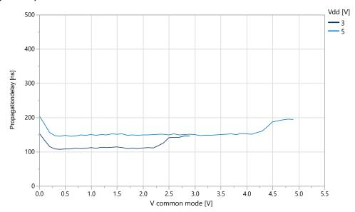
Figure 39-63. Propagation Delay vs.  $V_{CM}$  LPMODE Disabled, Falling Positive Input,  $V_{OD}$  = 30 mV (T=25°C)
