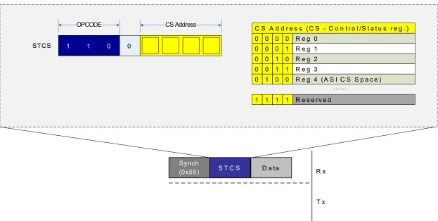
Figure 34-14 shows the data frame transmitted after the SYNCH and instruction frames. There is no response generated from the STCS instruction, as is the case for ST and STS.
