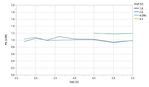
Figure 39-54. INL vs.  $V_{REF}$  ( $V_{DD}$ =5.0V,  $f_{ADC}$ =115 ksps, REFSEL = External Reference)
