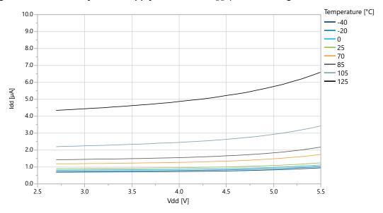
Figure 39-13. Standby Mode Supply Current vs. V<sub>DD</sub> (RTC Running with Internal OSCULP32K)
