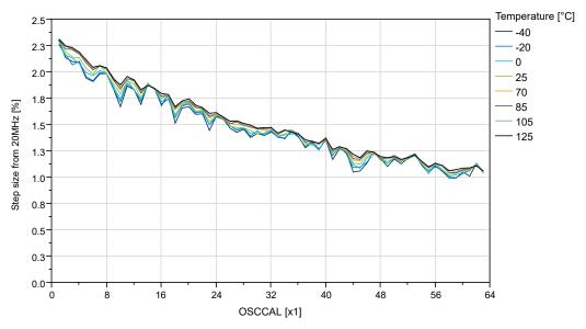
Figure 39-66. OSC20M Internal Oscillator: Frequency vs. Calibration Value (V<sub>DD</sub>=3V)
