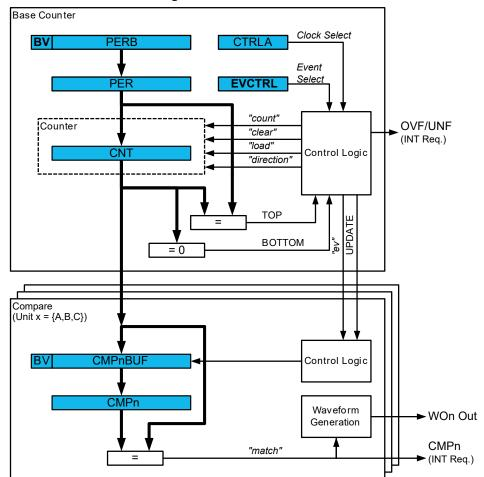
Figure 21-2. Timer/Counter Block Diagram
