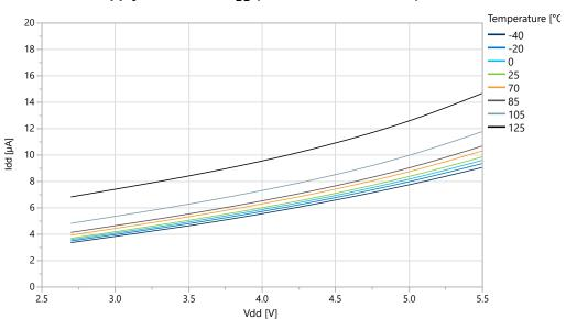
Figure 39-9. Idle Supply Current vs.  $V_{DD}$  (f=32 KHz OSCULP32K)
